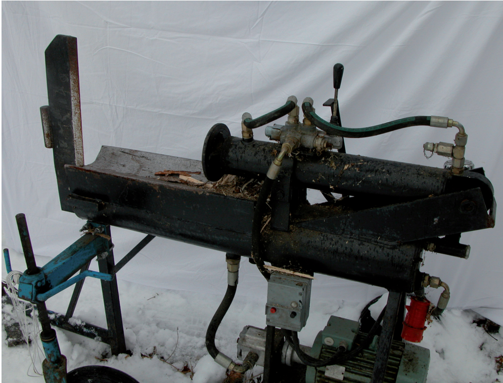
Figure 3. Home-made, lever controlled wedge splitter without warning notice or protective cover. Notes. Photography: Aron Lindqvist
