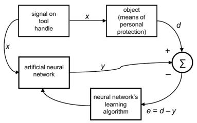
Figure 1. Identifying parameters of anti-vibration gloves with a neural network.
