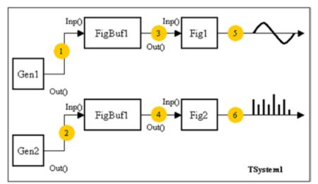
Figure 5. Sample system consisting of two signal generators and recorders for visualizing the runs at the outputs of the generators.
