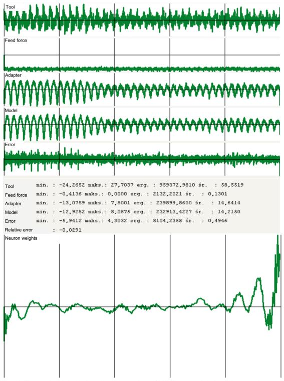
Figure 6. The results of simulation calculations: glove 8/drill 1/operator 3, 256 weights neural network, 128 weights neuron processing feed force.
