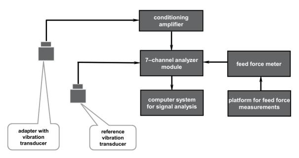
Figure 3. Measuring system for testing the vibration transmissibility of gloves.
