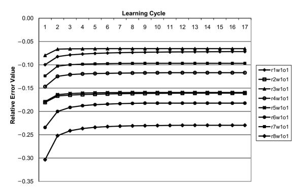
Figure 7. Changes in the value of the relative error when training a neural network simulating the behaviour of 8 gloves (r1-r8) for operator 1 (o1) using a drill (w1).
