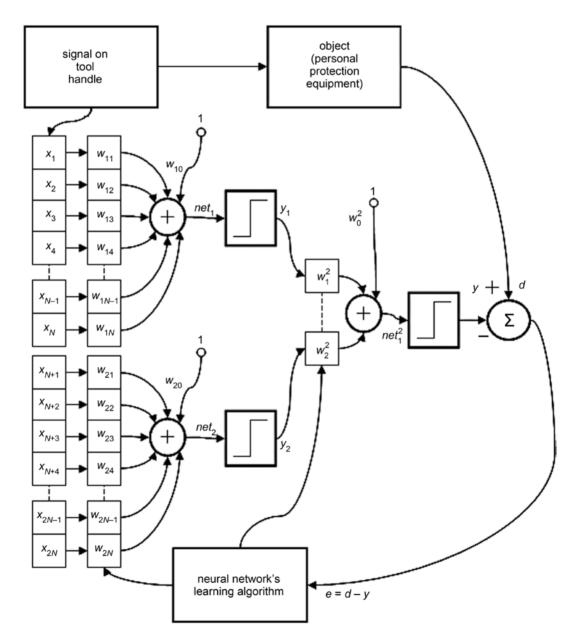
Figure 2. Identifying parameters of anti-vibration gloves with a multilayer, nonlinear neural network.
