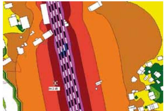
**Figure 3.** Map  $L_{day}$  calculated for a measurement point with SRM II [4]. Notes.  $L_{day}$ —A-weighted long-term average sound level as defined in Standard No. ISO 1996-2:2007 [37], determined over all day periods of a year.
